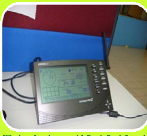
Wireless data logger with Davis Pro2 Console Display
