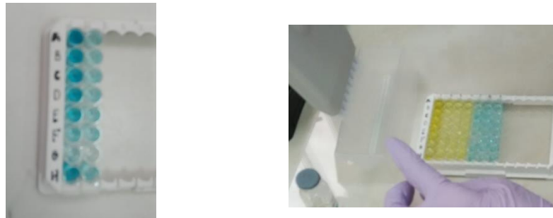
Figure 1. Color changing a) after addition of chromogen solution b) after addition of terminating solution
