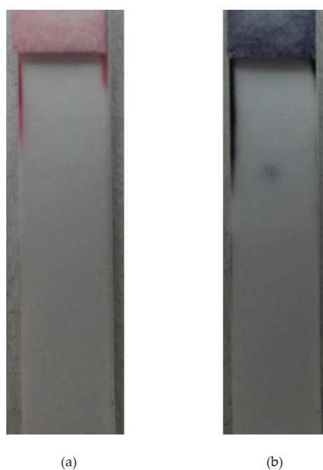
Figure 7. LFIA strips with control dot after flowed with conjugates of OD 2 for: (a) 40 nm AuNPs conjugate; (b) AuNFs conjugate.
