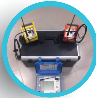
Water Pipe Leak Detector
