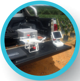
Phantom 4 Pro equipped with Multispectral camera
