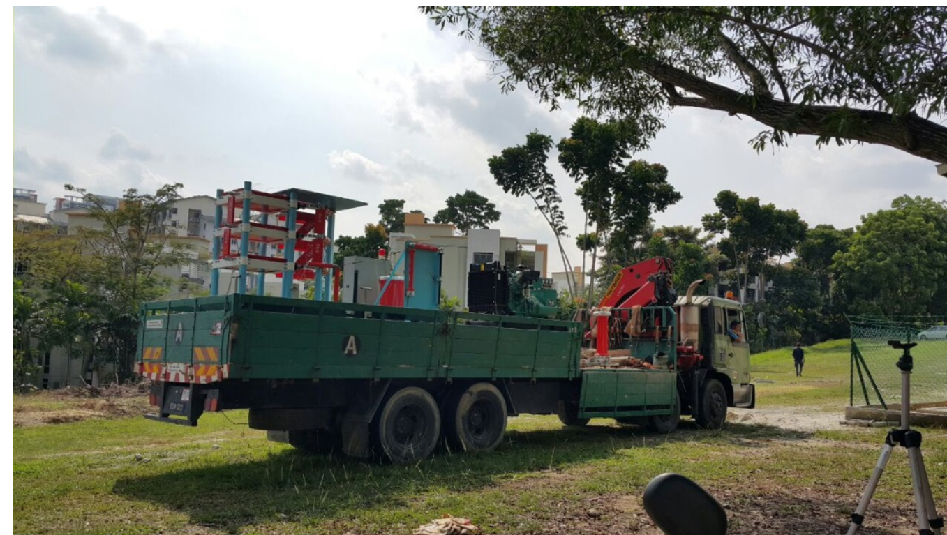
The HV equipment can be mounted on a lorry for field measurements.
