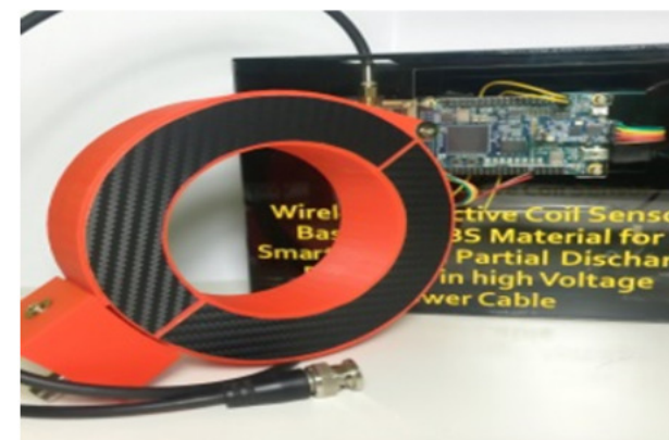
Wireless inductive coil sensor made from ABS for PD detections.
