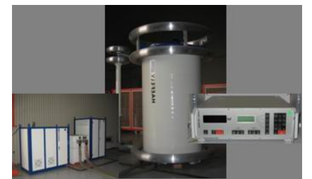
250 kV HVAC test set.
