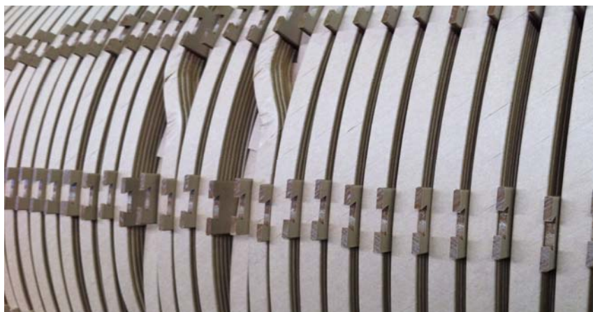
Solid insulators: paper and pressboard insulation.
