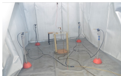
Power frequency withstand wet test.
