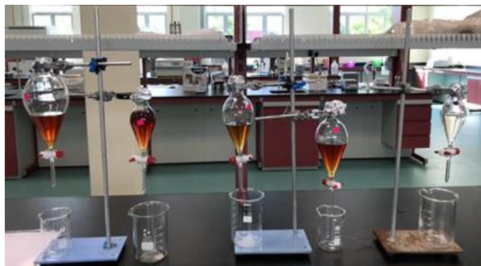
Figure 3: Biodiesel (up layer) and glycerine (bottom layer) were separated by using separating funnel.
