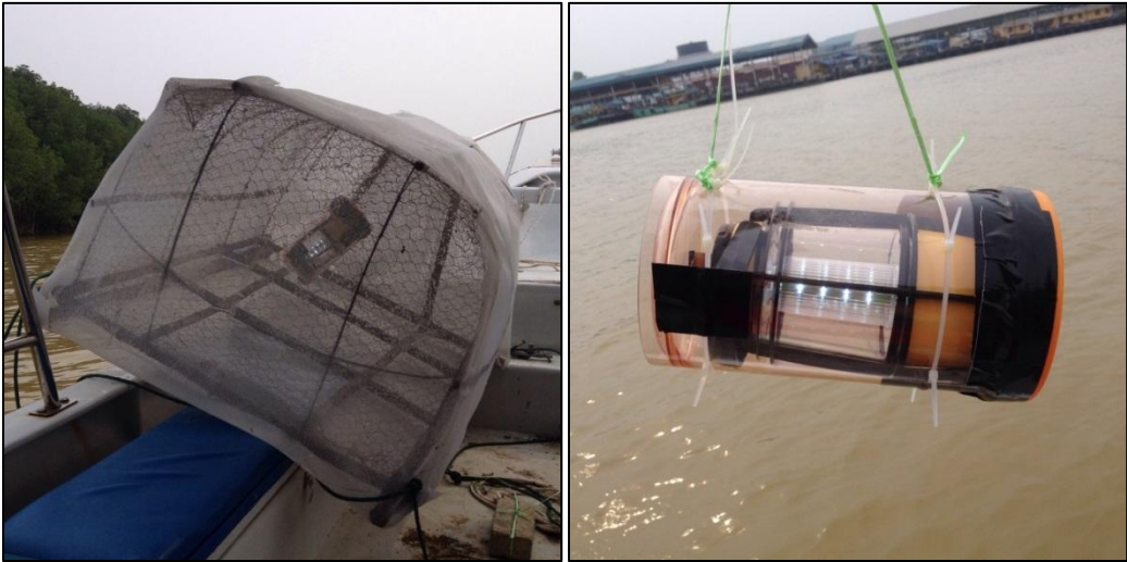
Figure 2: Modified bubu light trap and the prepared internal light source used to attract the Ichthyoplankton during sampling.
