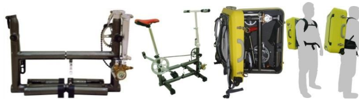
Figure 3: Portable body frame and case design.
