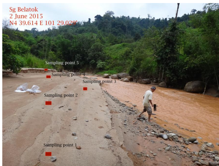
Figure 1: Example of sampling strategy for sediment samples along riverbanks for sediment fingerprinting analysis.
