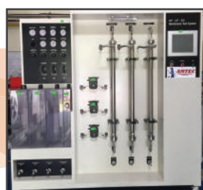
Industrial Lab Scale Hybrid MF + UF + RO Membrane Testing system
