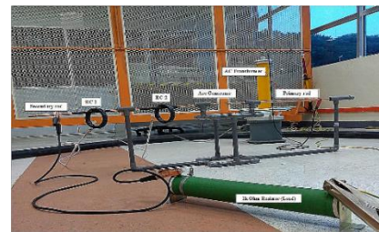
Figure 2: Indoor Modelling of Series Arcing Fault and Setup in the High voltage lab
