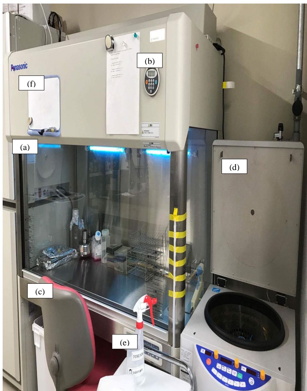
Figure 3.3 Workstation for cell culture consisted of (a) biological safety cabinet for cell culture, (b) time counter, (c) chair, (d) centrifuge, (e) alcohol, and (f) white board. See appendix B for list of equipment and appliances used.
