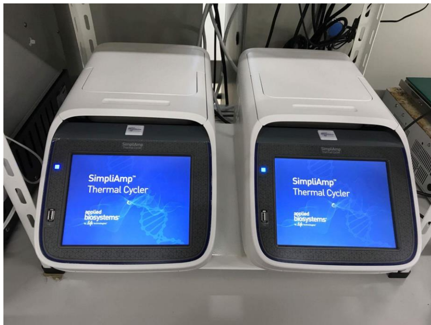
Figure 3.9 Thermal cycler device for cDNA conversion. See appendix B for specifications of thermal cycler.
