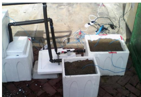
Chilled Water Tanks, Cooled Soil bed, and Controlled Soil Bed
