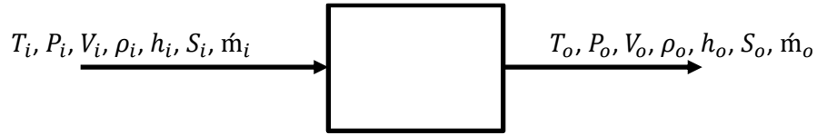
Figure 3.10: Component energy balance model
