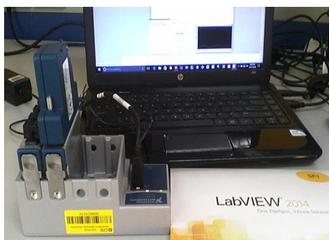
NI and LabVIEW Installations for Data Logging
