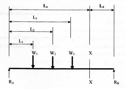
Shear force at section X - X is:
