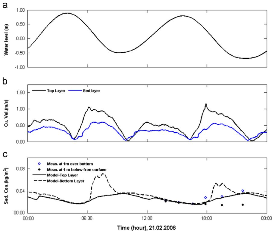
**Fig. 7.** Computed and measured sediment concentrations near the bed and below the free surface at Station L- for spring tidal cycle from 21 February 2008. Also shown are measured depths and computed velocities.
