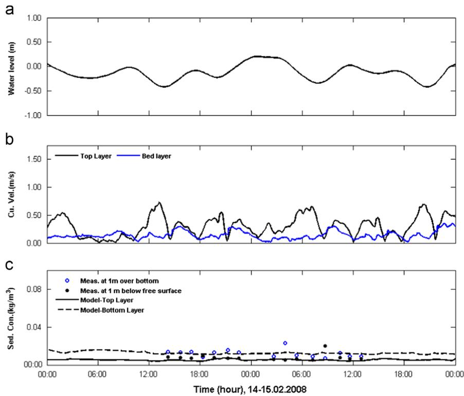
**Fig. 6.** Computed and measured sediment concentrations near the bed and below the free surface at Stations L- for neap tidal cycle from 14 to 15 February 2008. Also shown are measured depths and computed velocities.
