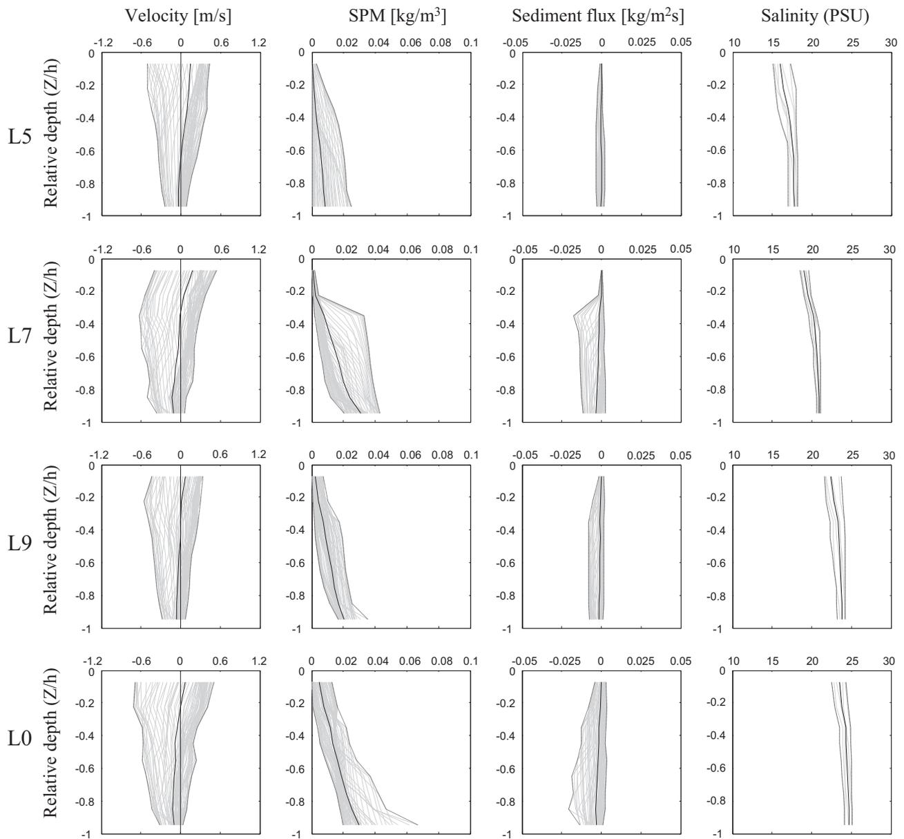
**Fig. 11.** Depthwise variations of computed velocity, suspended sediment concentration and salinity along the navigation channel for neap tidal cycle on 5th of September 2007.
