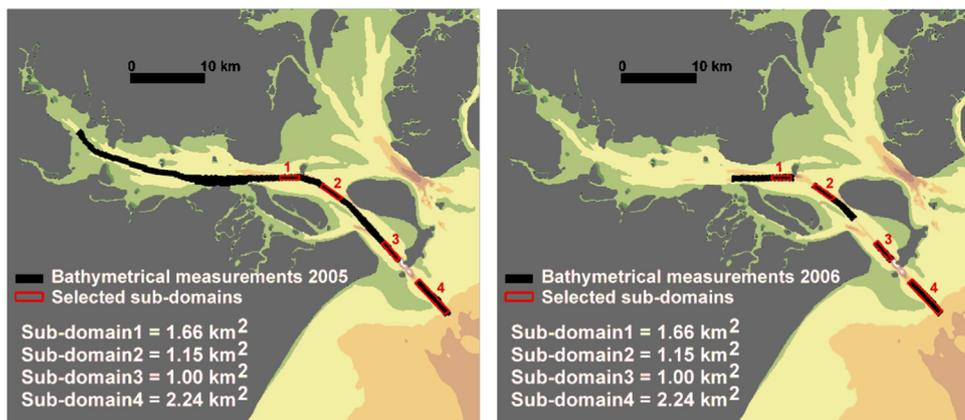
Fig. 13. Location of bathymetrical surveys and selected sub-domains – 2005 (left) and 2006 (right).
