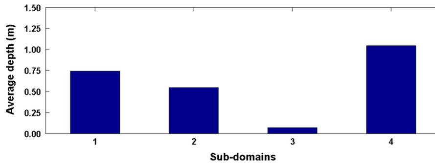
Fig. 14. Mean bed elevation changes from 2005 to 2006 at Stations 1 to 4.
