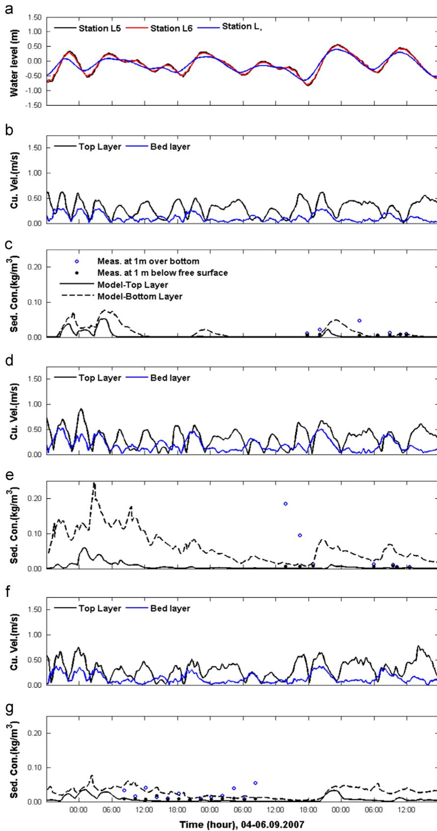
Fig. 4. Computed and measured sediment concentrations near the bed and below the free surface at Stations L5, L6 and L- for neap tidal cycle from 4 to 6 September 2007. Also shown are measured depths and computed velocities.
