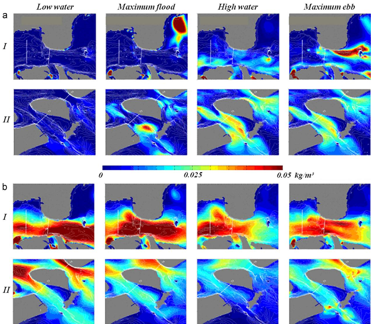
Fig. 10. Distribution of suspended sediment concentration at top layer of depth during neap and spring tides.
