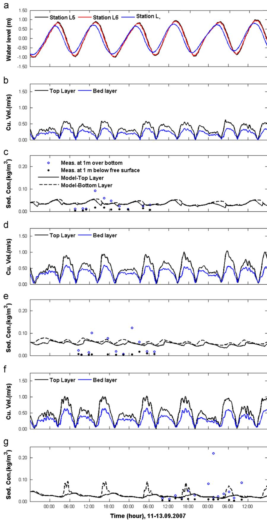
Fig. 5. Computed and measured sediment concentrations near the bed and below the free surface at Stations L5, L6 and L- for spring tidal cycle from 11 to 13 September 2007. Also shown are measured depths and computed velocities.
