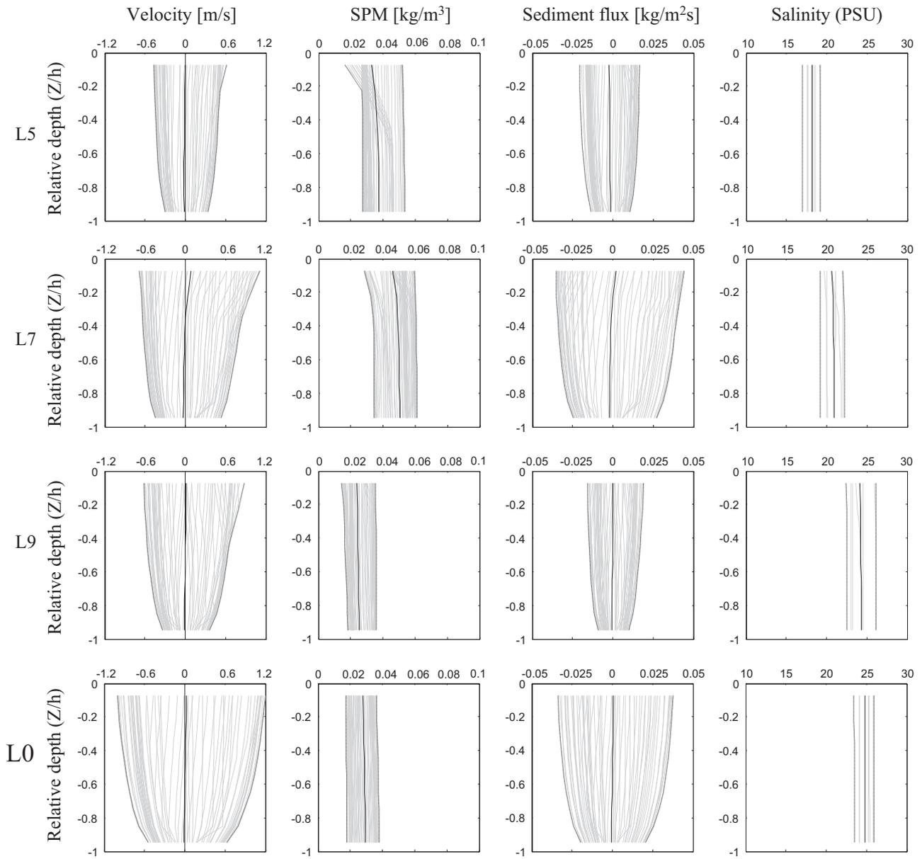
Fig. 12. Depthwise variations of computed velocity, suspended sediment concentration and salinity along the navigation channel for spring tidal cycle on 13 September 2007.
