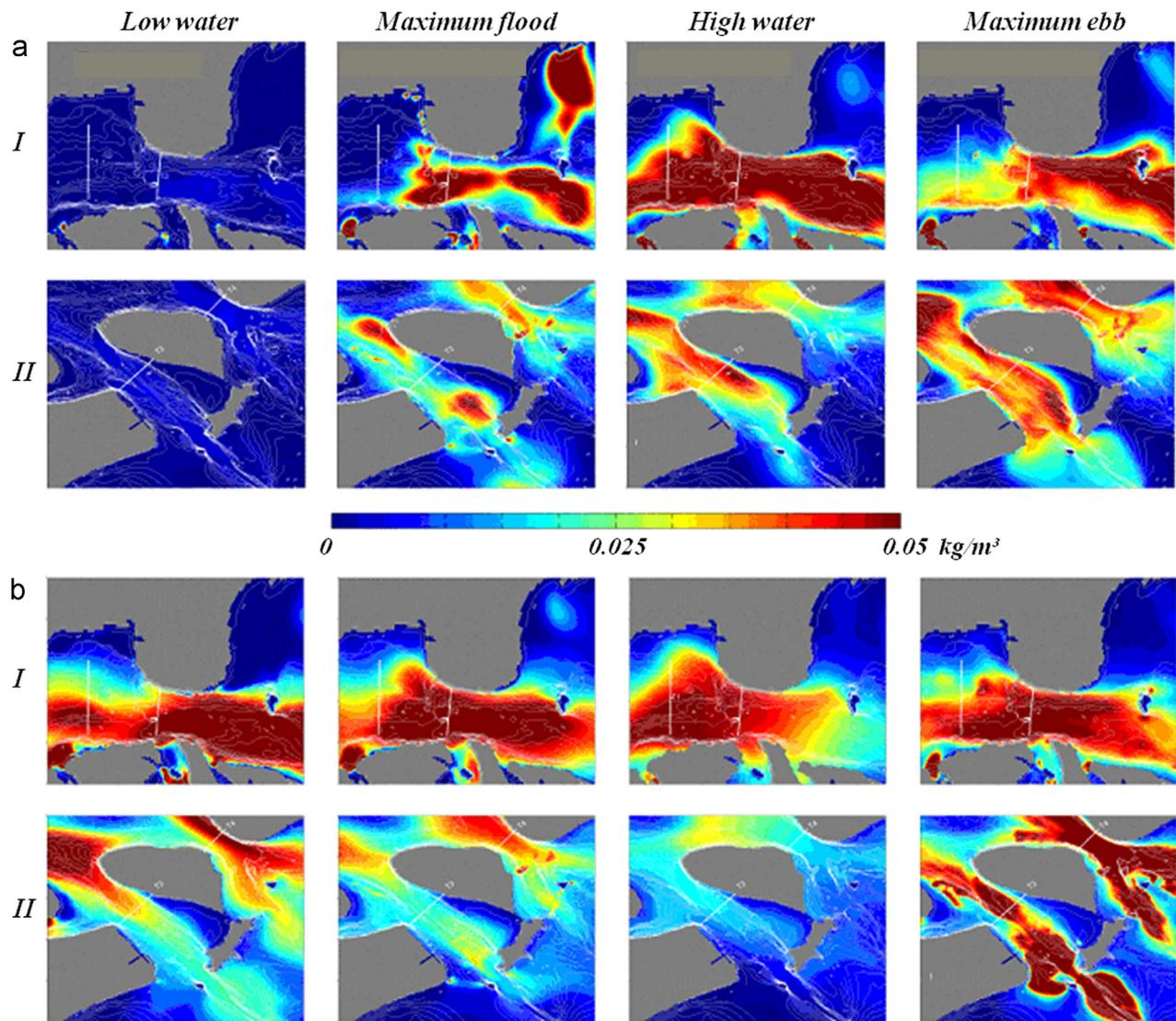
Fig. 9. Distribution of suspended sediment concentration at the *bottom layer* of depth during neap and spring tides.
