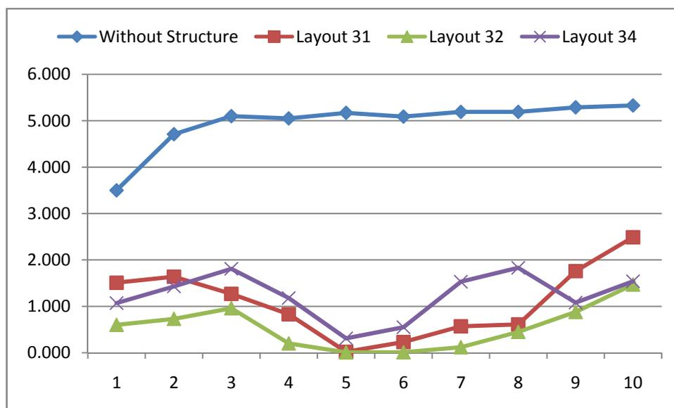
**Figure 5.7** Attenuation of Tsunami Wave Height on the Shoreline for Without Structure and With Layouts 31, 32 and 34 Conditions.
