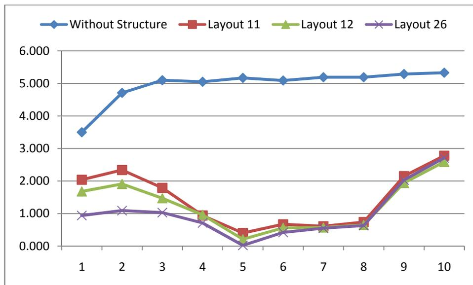
**Figure 5.6** Attenuation of Tsunami Wave Height on the Shoreline for Without Structure and With Layouts 11, 12 and 26 Conditions.
