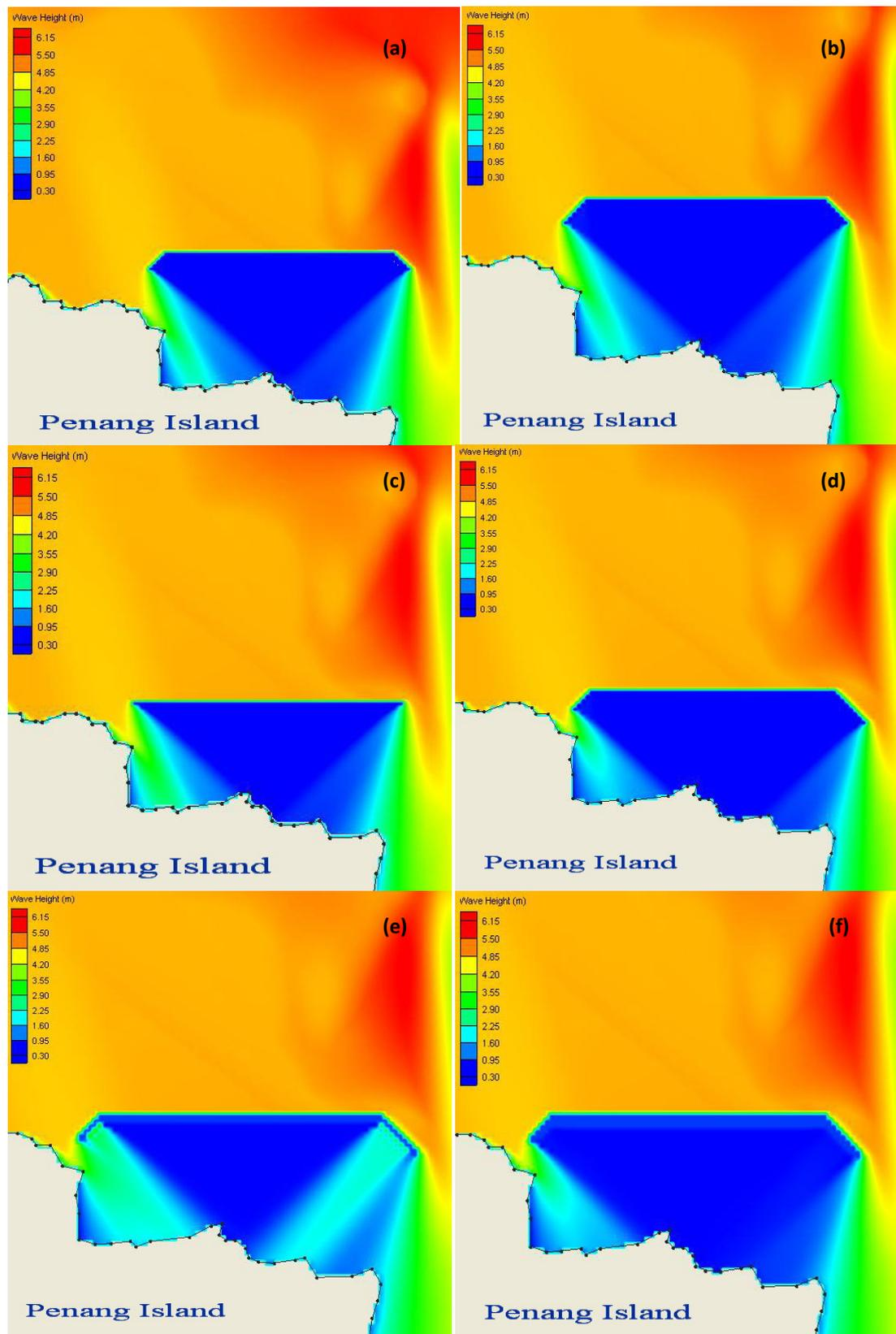
**Figure 5.4** Distribution of Wave Height on the Shoreline Due to the Presence of
