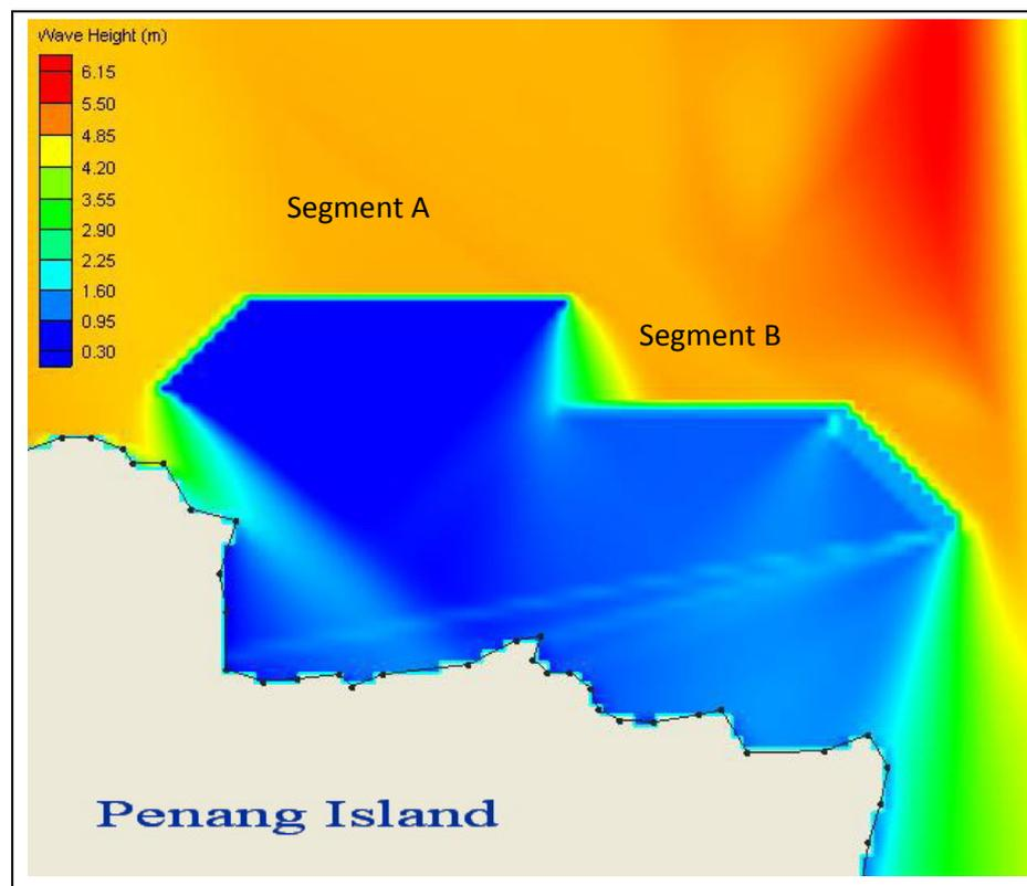
**Figure 5.13** Distribution of Tsunami Wave Heights on the Shoreline with the Construction of Breakwater Layout 39
