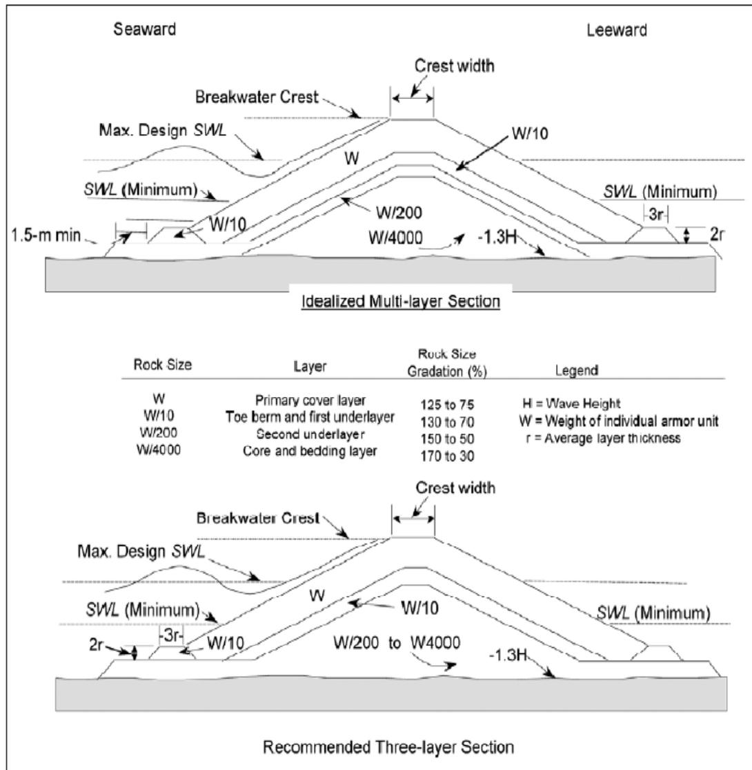
**Figure 3.3** Rubblemound Section for Seaward Wave Exposure with Zero-to-Moderate Overtopping Conditions (Source: USACE 2006)
