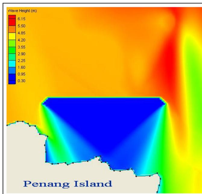
**Figure 5.3** Distribution of Wave Height along the Shoreline Due to the Presence of Breakwater with Two Arms.
