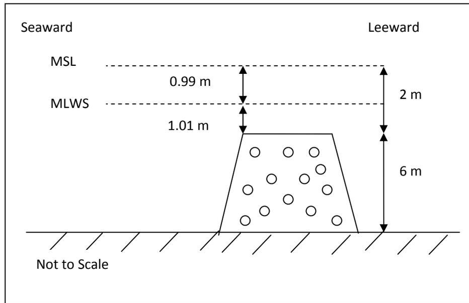
**Figure 5.12** Cross Section of Segment B for Layout No.39
