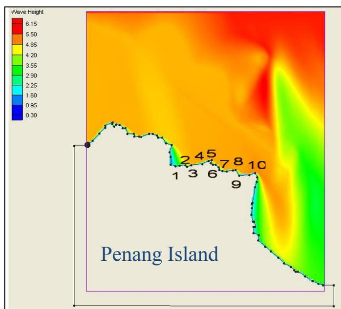
**Figure 5.1** Typical Outputs of Wave Heights Generated By STWAVE for the Existing Condition Without Any Structure
