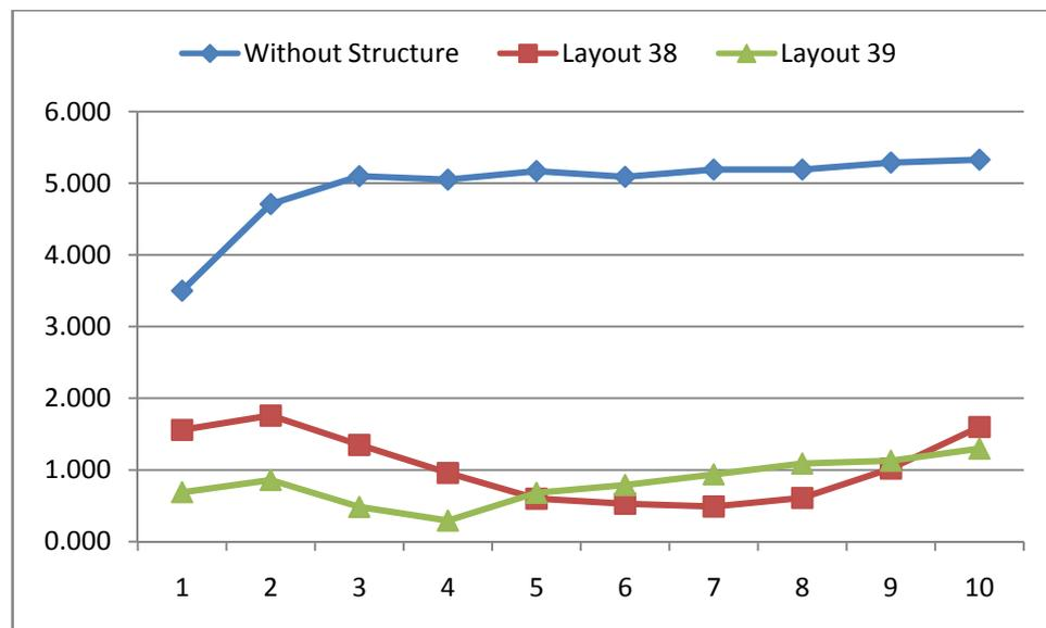
**Figure 5.9** Attenuation of Tsunami Wave Height on the Shoreline for Without Structure and With Layouts 38 and 39 Conditions.
