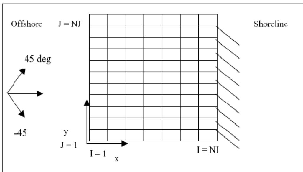
**Figure 3.5** Schematic Grid of STWAVE (Source: Smith et al 2001)
