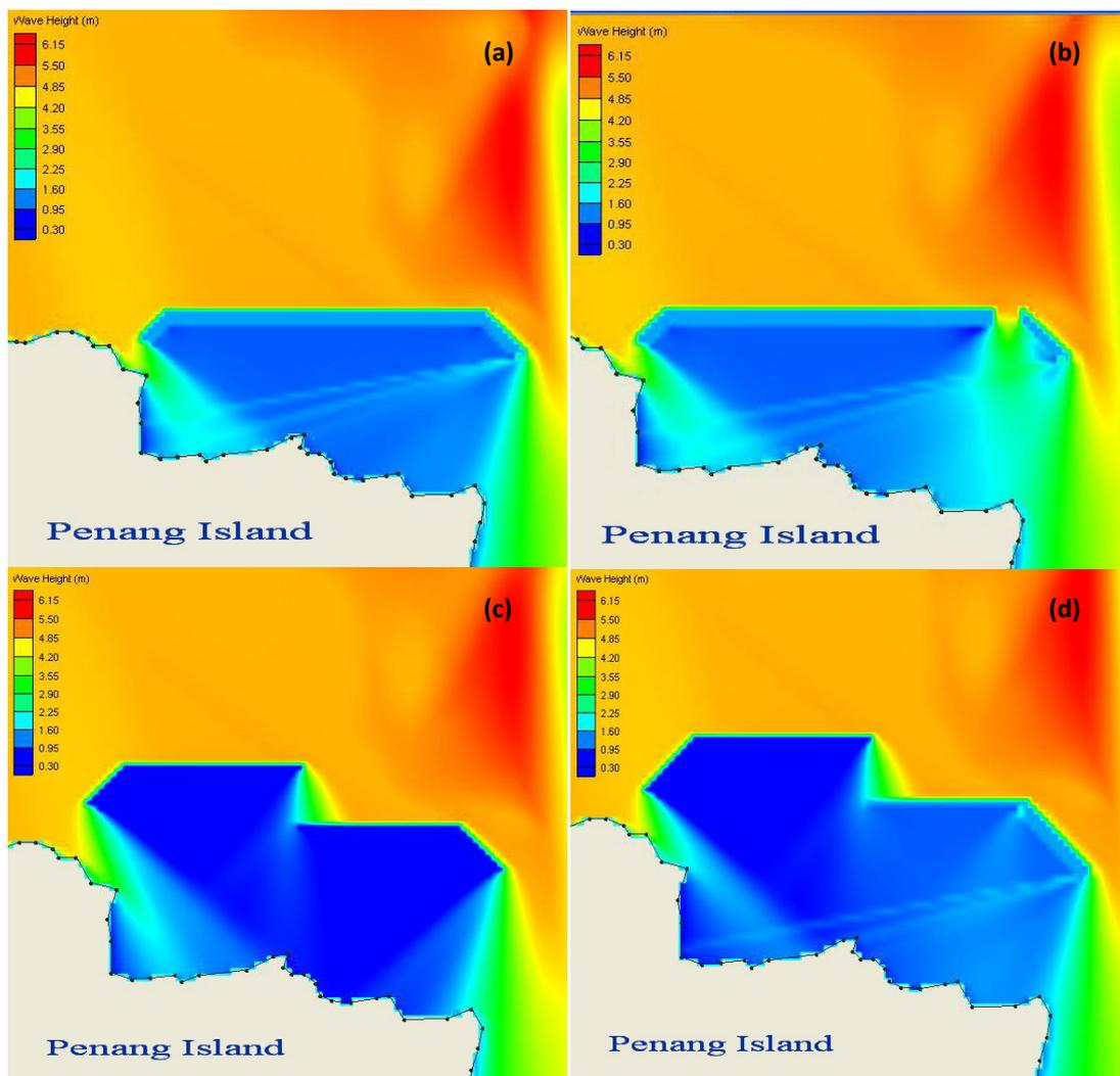
**Figure 5.5** Distribution of Wave Height on the Shoreline Due to the Presence of (a) Layout 36 (b) Layout 37 (c) Layout 38 (d) Layout 39
