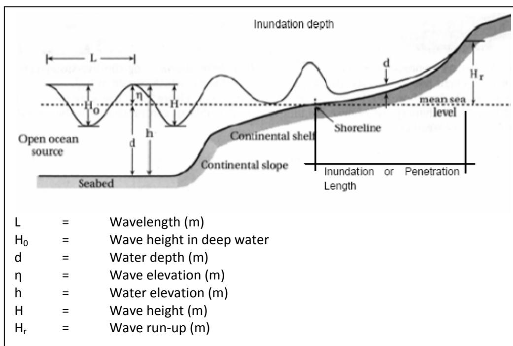
**Figure 2.1** Terminology of Tsunami Waves (Source: Van der Plas 2007)
