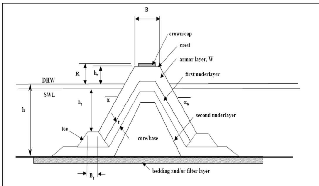
**Figure 3.2** Parameters used in Rubblemound Design (Source: Sheppard 2004)
