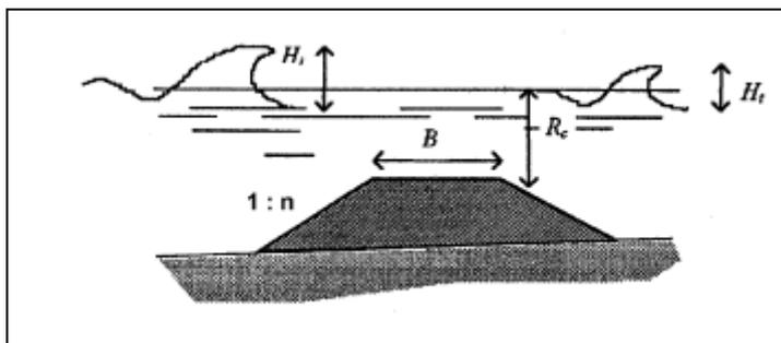
**Figure 2.7** Wave Reduction Caused by a Submerged Structure
