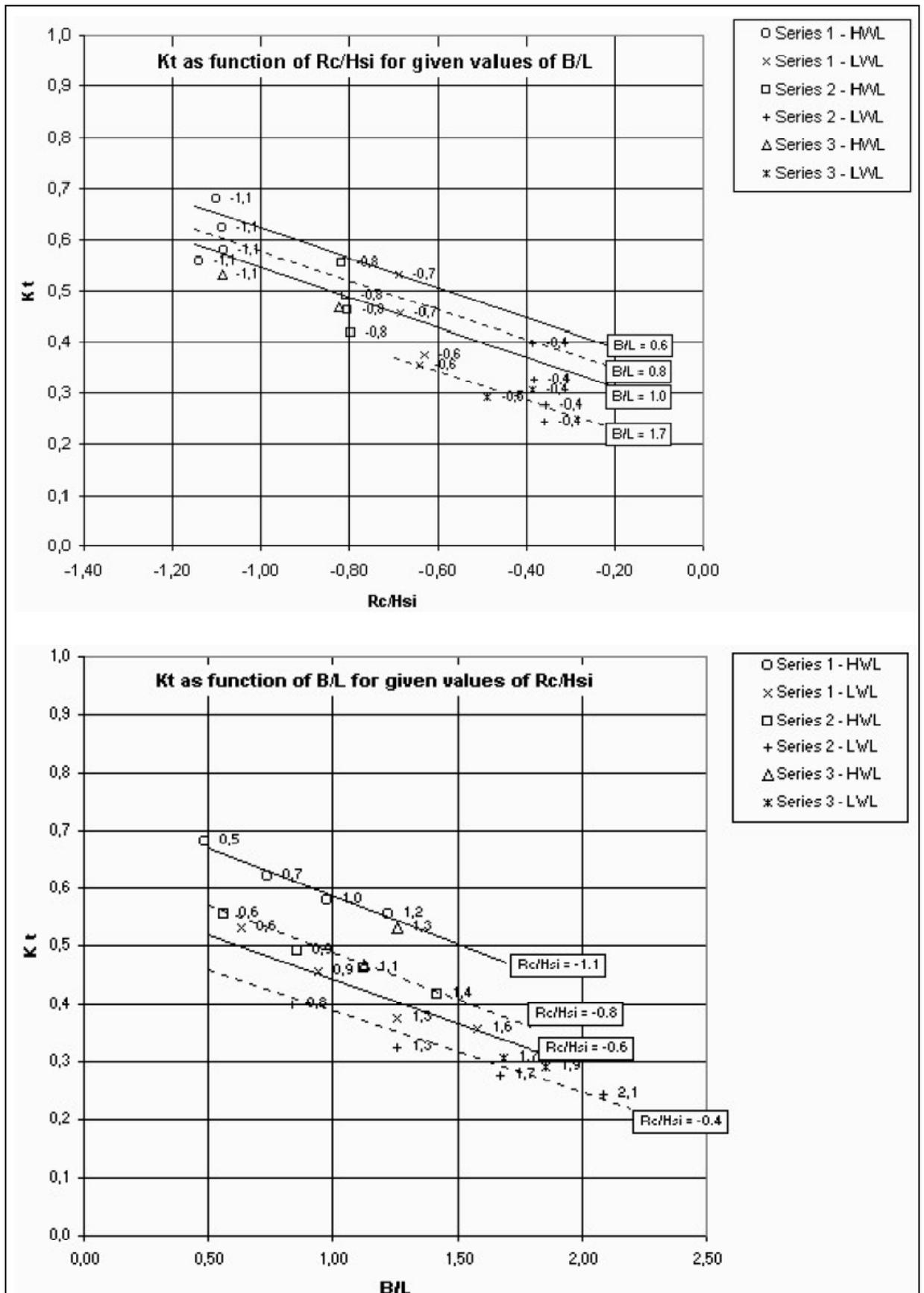
**Figure 2.8** Wave Transmissions over Reef Structures in Amwaj Project (Source: Pilarczyk 2003)
