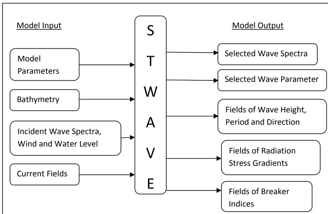
**Figure 3.6** Schematic Input/Output Files of STWAVE
