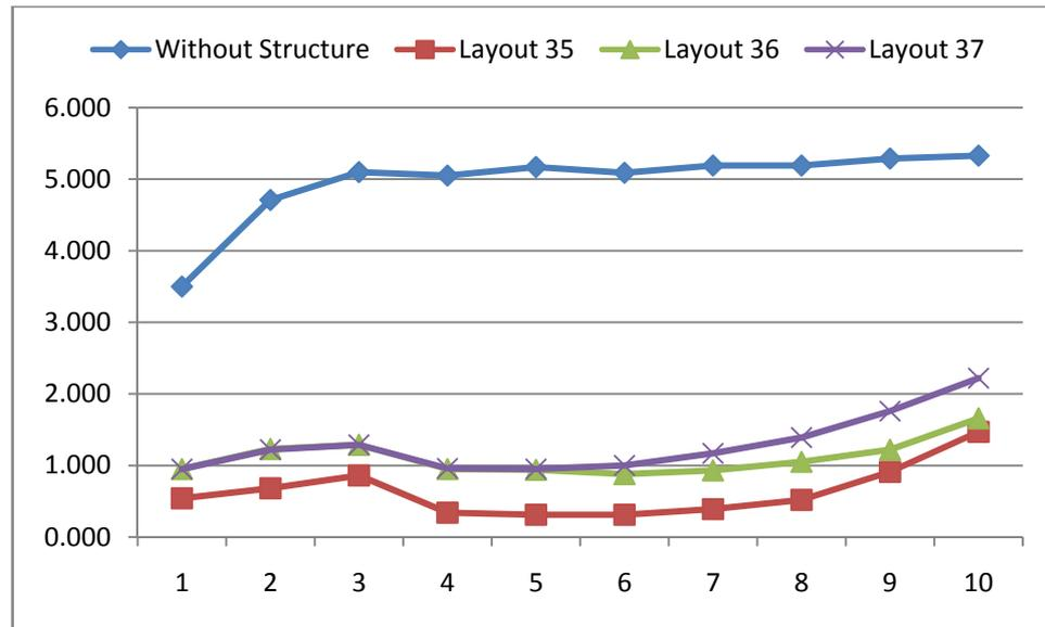
**Figure 5.8** Attenuation of Tsunami Wave Height on the Shoreline for Without Structure and With Layouts 35, 36 and 37 Conditions.
