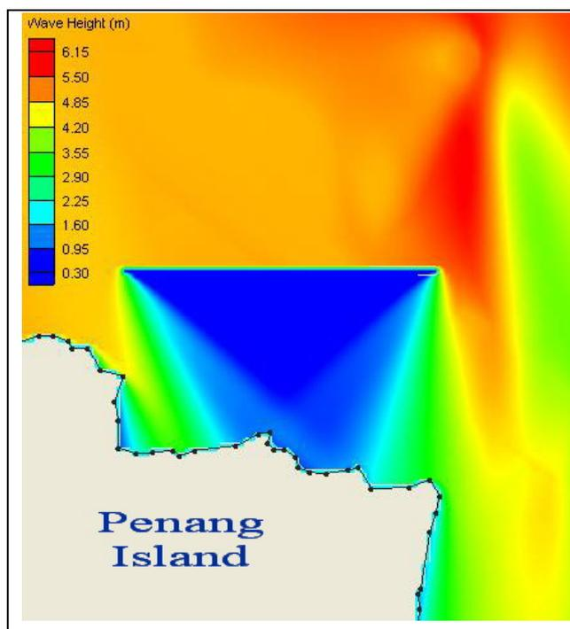
**Figure 5.2** Distribution of Wave Height on the Shoreline Due to the Presence of Breakwater Layout 1
