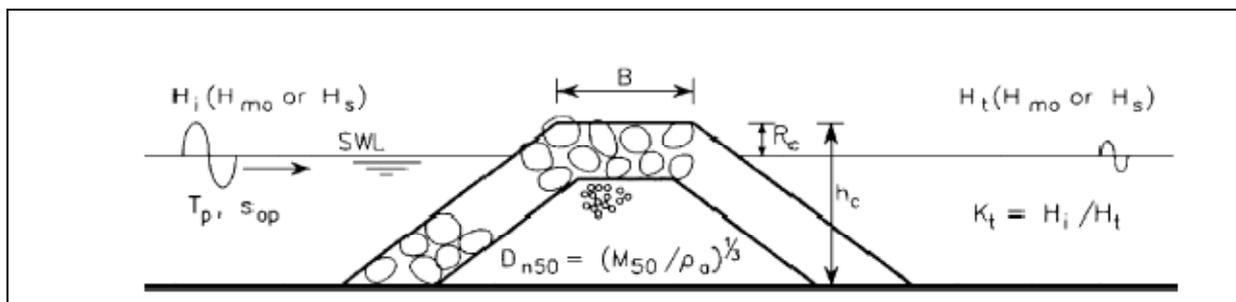
**Figure 2.10** Definitions of Governing Parameters Involved in Wave Transmission through LCS (Source: Van der Meer et al 2005)
