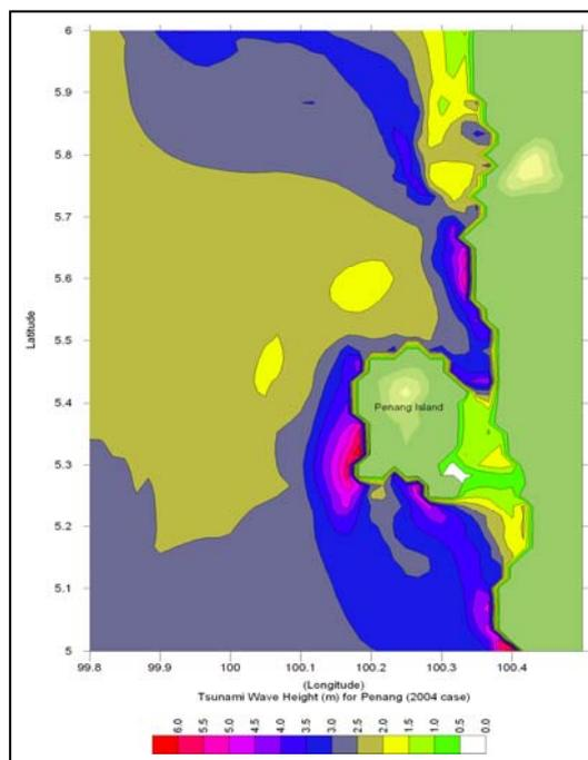
**Figure 4.2** Offshore Tsunami Wave Height Generated Using TUNAMI N2
