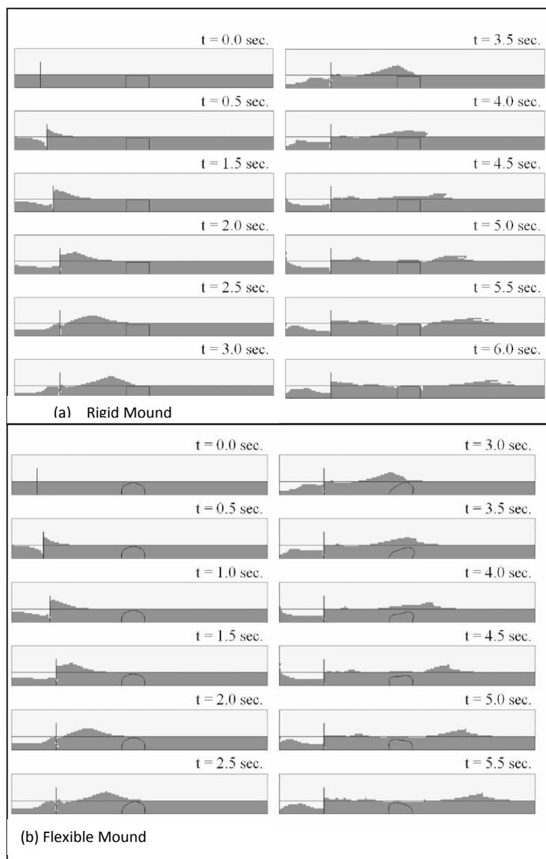
**Figure 2.9** Wave Propagation Passing Over (a) Rigid Mound (b) Flexible Mound
