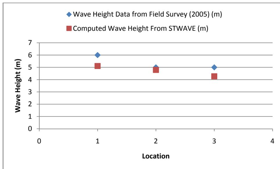
**Figure 4.16** Plot Showing Observed and Computed Wave Heights at the Location Points
