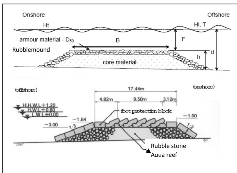
**Figure 2.11** Typical Armour Type for Submerged Breakwater Used in Van der Meer et al’s Research Works (Source: Pilarczyk 2003)
