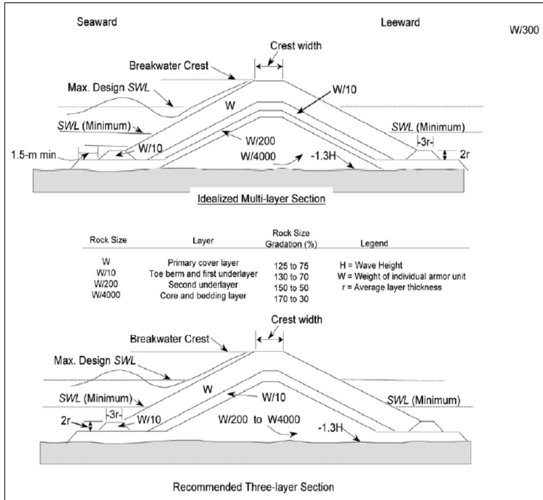
**Figure 3.4** Rubblemound Section for Wave Exposure on Both Sides with Moderate Overtopping Conditions (Source: USACE 2006)
