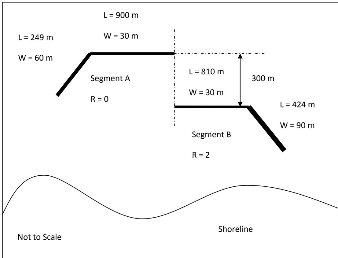
**Figure 5.10** Plan of the Optimized Breakwater for Layout No.39
