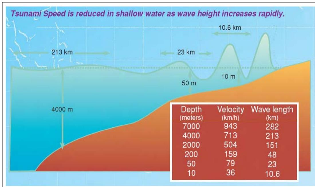
**Figure 2.6** Typical Changes in Tsunami Wave as it Reaches Shallow Water
