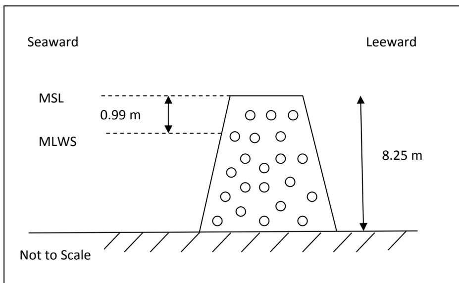
**Figure 5.11** Cross Section of Segment A for Layout No.39
