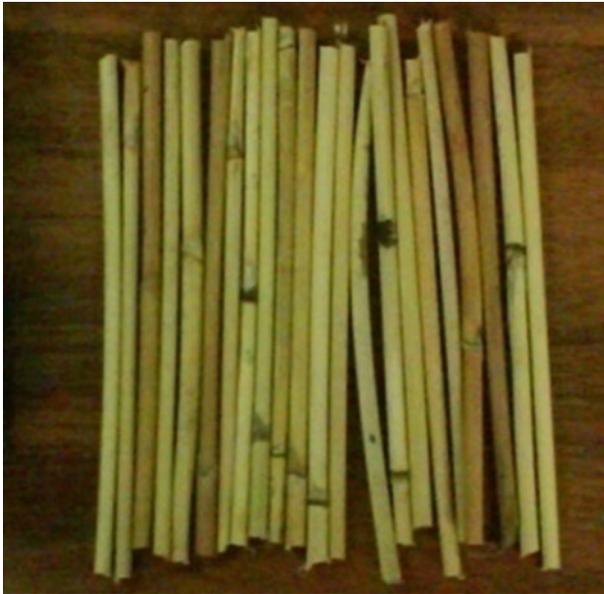
**Fig. 8** The rattans after being cut into 20 cm lengths
