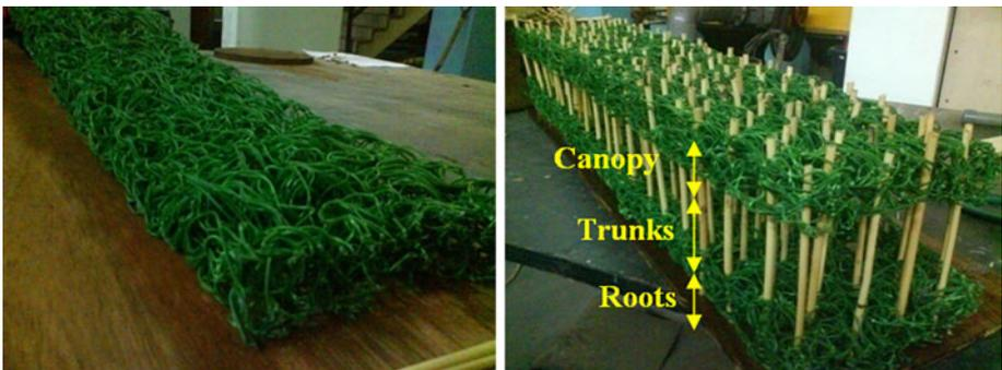
**Fig. 5** Plastic porous material representing the model tree canopy
