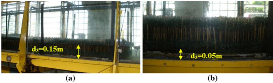
**Fig. 9** Water-level settings; (a) High water and (b) Low water
