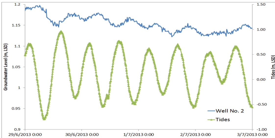
Figure 6. Groundwater table in well no. 2 and tidal elevation
