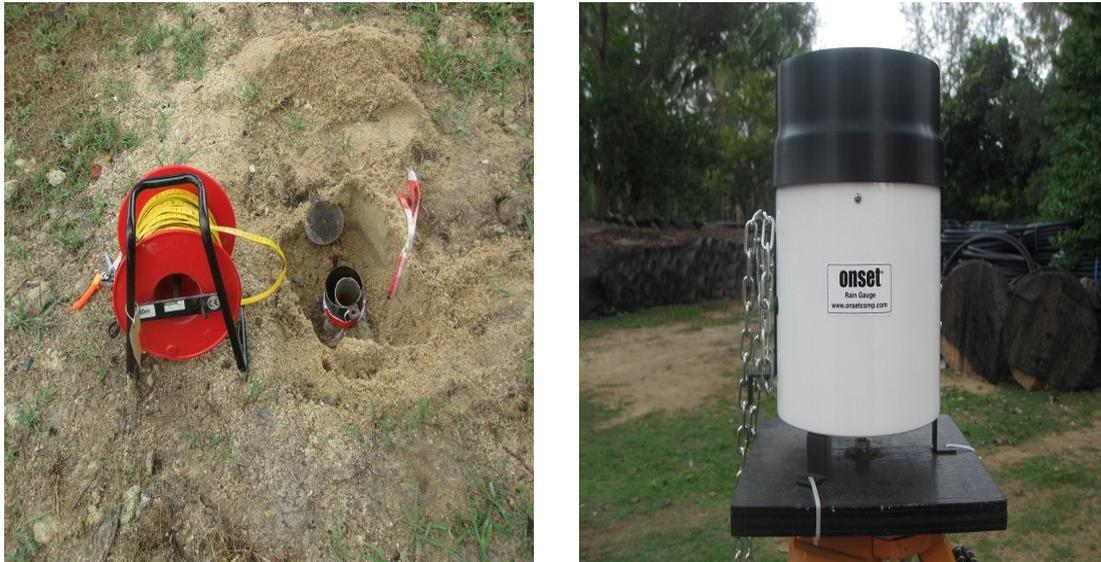
**Figure 4. Photograph showing the (left) monitoring well with water level indicator and (right) rain gauge station**
