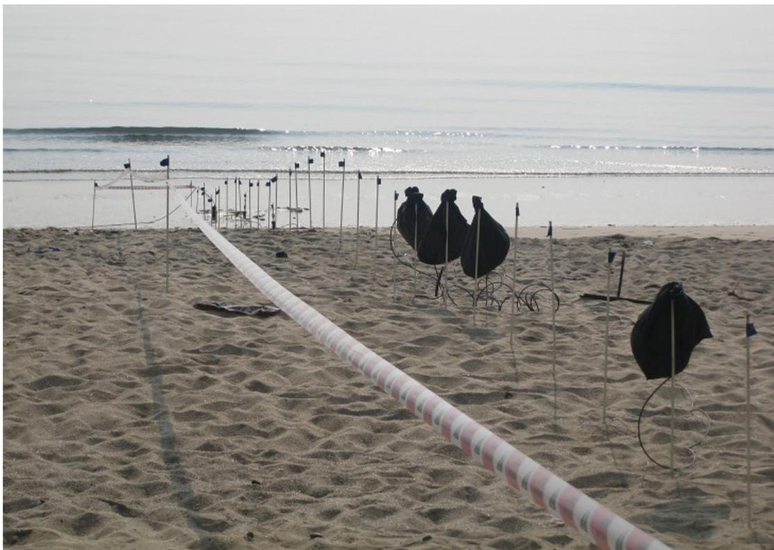
Figure 2. Photograph showing the steel rods were installed cross section with spacing 1 meter at Desaru beach
