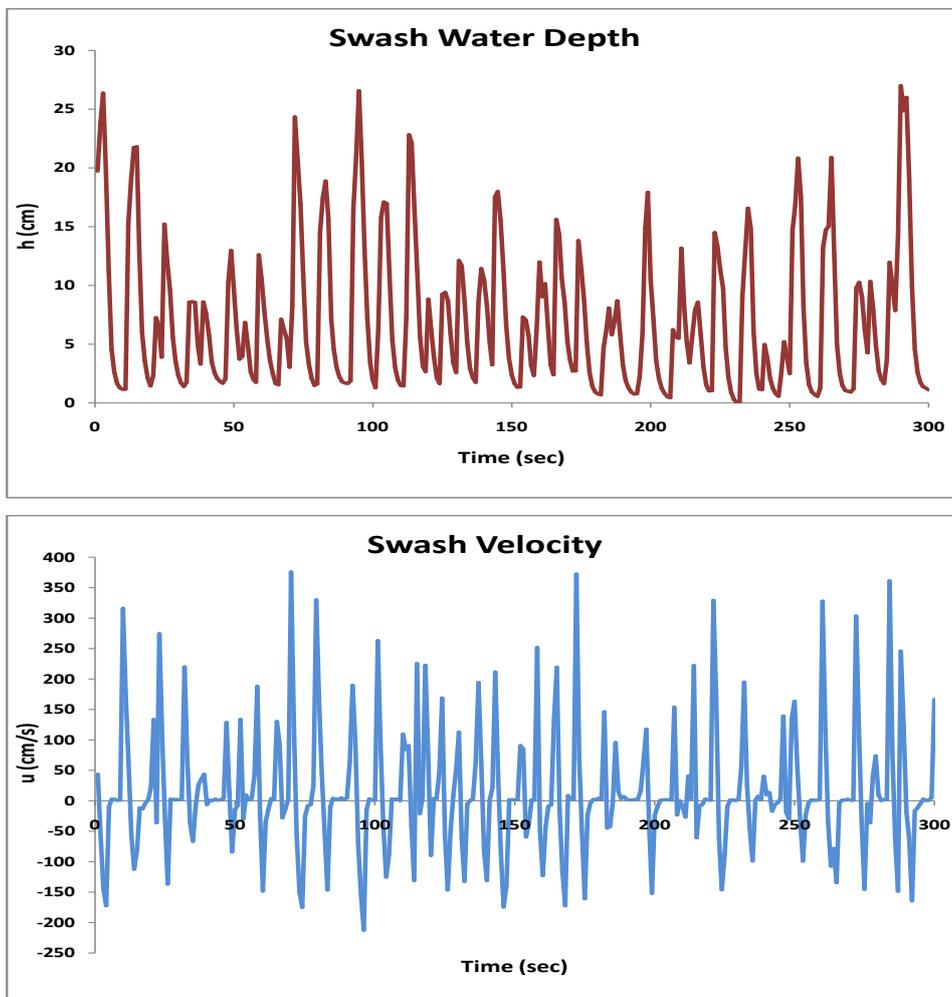
Figure 7. Profiles of swash water depth and velocity during wet season
