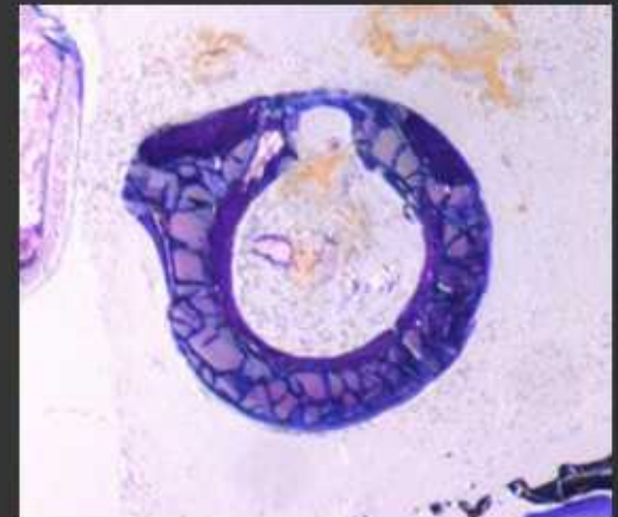
Transformation of a MAGNEZIX® Compression Screw into calcium phosphate after 12 months with clear bone adsorption.
