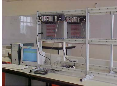
Figure 3. PLCs integration through network.
