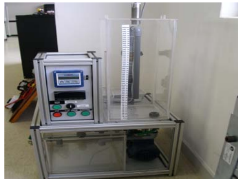
Figure 6. Plant 3 - Water Level System
