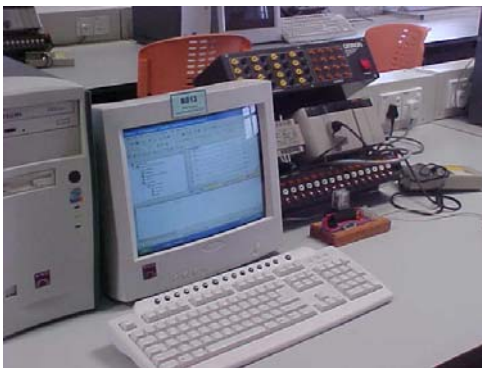
Figure 2. PC is used for uploading/downloading program using PLC's software tools.
