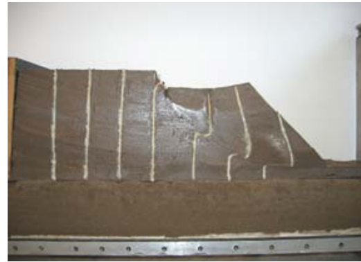
Fig. 4 Example of a failed slope tested in a centrifuge [9].
