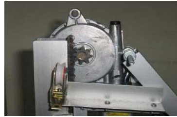
Fig. 13. Track power windows motor.
