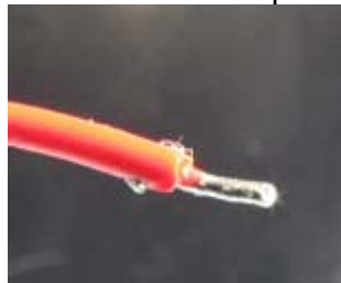
Stripped wire end
