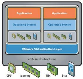
Fig.2. x86 Architecture after Virtualization [2]
