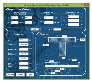
Figure 1. Elastic Deflection of a cantilever beam (2007)
