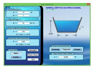
Figure 3. Normal Depth of an Open Channel (2010)
