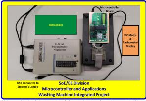
Figure 4 depicts a standalone In-circuit microcontroller programmer along with a purposefully designed and customized circuit board with INTEL 8051 microcontroller.
