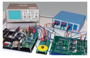
Figure 6. Hardware set-up of a servo control motor set
