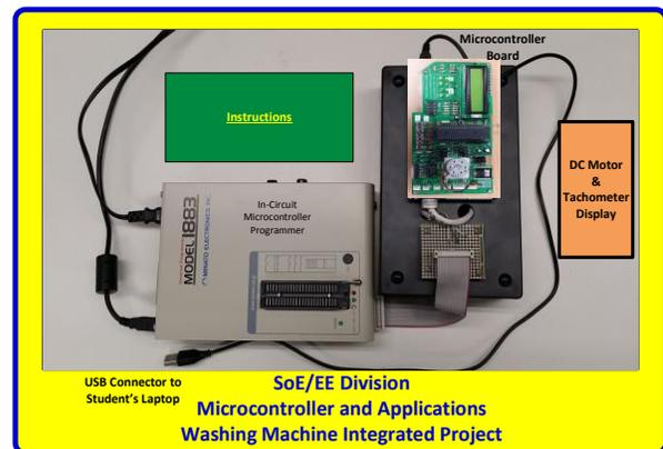
Figure 4 depicts a standalone In-circuit microcontroller programmer along with a purposefully designed and customized circuit board with INTEL 8051 microcontroller.
